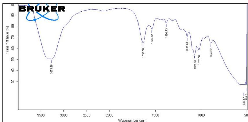
Figure 2: FTIR analysis of chitosan nanoparticle.
