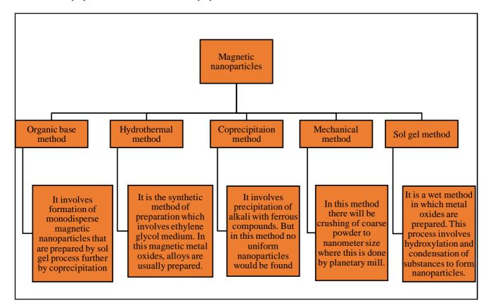
Figure 2: Method of preparation of MNPs, 1. Organic base method; 2. Hydrothermal method; 3. Coprecipitation method; 4. Mechanical method; 5. Sol-gel method.
