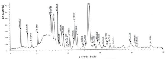
[] File: XRPD-839 raw - Start: 2.0000 \* - End: 50.0014 \* - Step: 0.0053 \* - Step time: 13.9 s - Anode: Cu - WL1: 1.5406 - Creation: 05.04.2019 13:13:40
